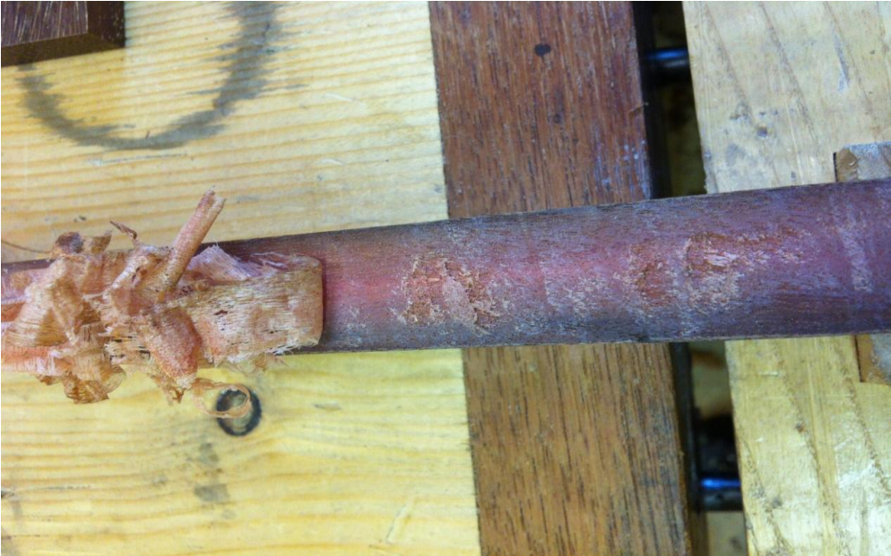
Figure 3 Lignum vitae with deep tearout while taking a light shaving
